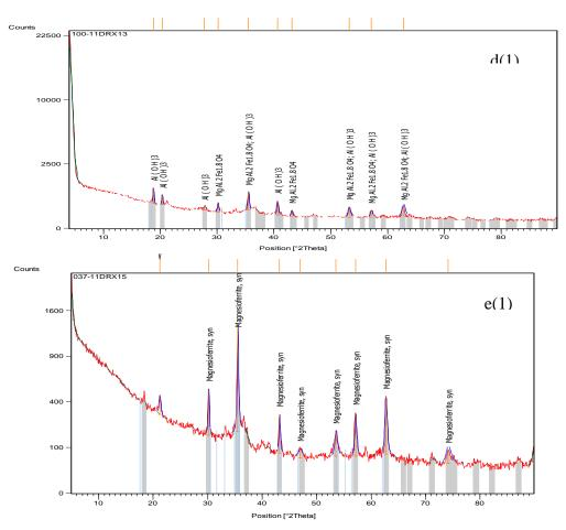
**Figure 1:** Chemical composition of the adsorbents-coagulants prepared in neutral medium. a(1): 100%Al/0%Fe (N1); b(1): 75%Al/25%Fe (N2); c(1): 50%Al/50%Fe (N3); d(1): 25%Al/75%Fe (N4); e(1): 0%Al/100%Fe (N5).
