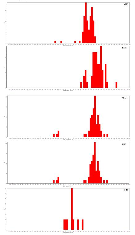
**Figure 2:** Zeta potential of colloids particles of the adsorbents-coagulants prepared in neutral medium. a(2): 100%Al/0%Fe (N1); b(2): 75%Al/25%Fe (N2); c(2): 50%Al/50%Fe (N3); d(2): 25%Al/75%Fe (N4); e(2): 0%Al/100%Fe (N5).
